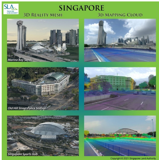
Caption: Singapore Land Authority captured more than 160,000 high-resolution aerial images over a 41-day period and selected ContextCapture to process them into a 0.1-meter accurate nationwide 3D reality mesh.
