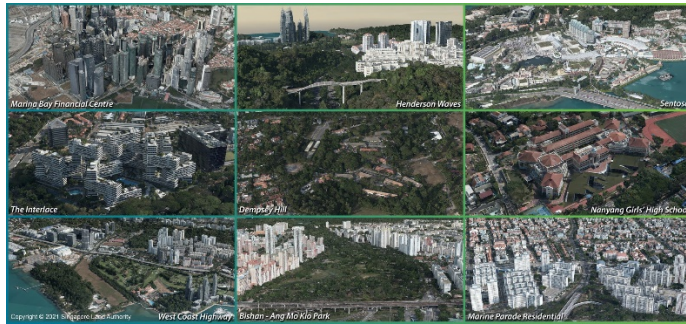
Caption: In 2019, Singapore Land Authority initiated a second mapping to detect the changes over time and update a mapping created in 2012 with improved accuracy to reflect the country's dynamic urban development. The project required aerial mapping of the entire country, and mobile street mapping of all public roads in Singapore.
