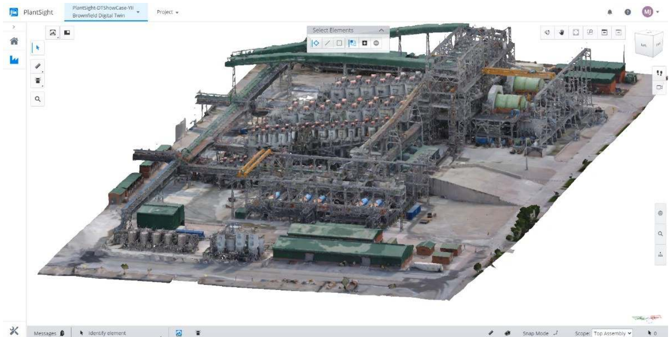
Bentley's Context Capture software creates a reality model, a quick way to start building a 3D digital twin.
